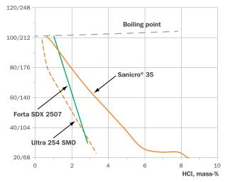
Fig. 1. Preliminary isocorrosion diagram for Sanicro® 35 in hydrochloric acid. The line represents a limit, below which the corrosion rate is expected to be lower than 0.1 mm/year. Other grades are included for comparison.
